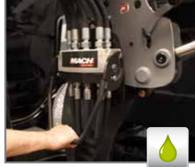
MACH System® - "non drip" instant coupling of tractor to loader hydraulic and electric lines.
