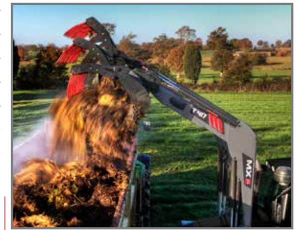
Unrivalled dump speed and optimum crowd angles thanks to a unique asymmetric ram design.
