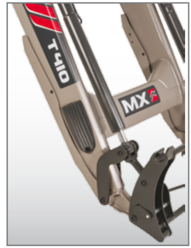
Fully protected parking stands integrated into the loader arms. The lift height remains unchanged.
