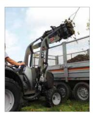
MAXIMUM LIFT HFIGHT AND REACH One of the main attributes of MX COMPACT loaders is maintaining the compactness of the tractor/loader units, whilst acheiving the maximum lift height and reach to easier dump materials into high trailers and stack pallets.
