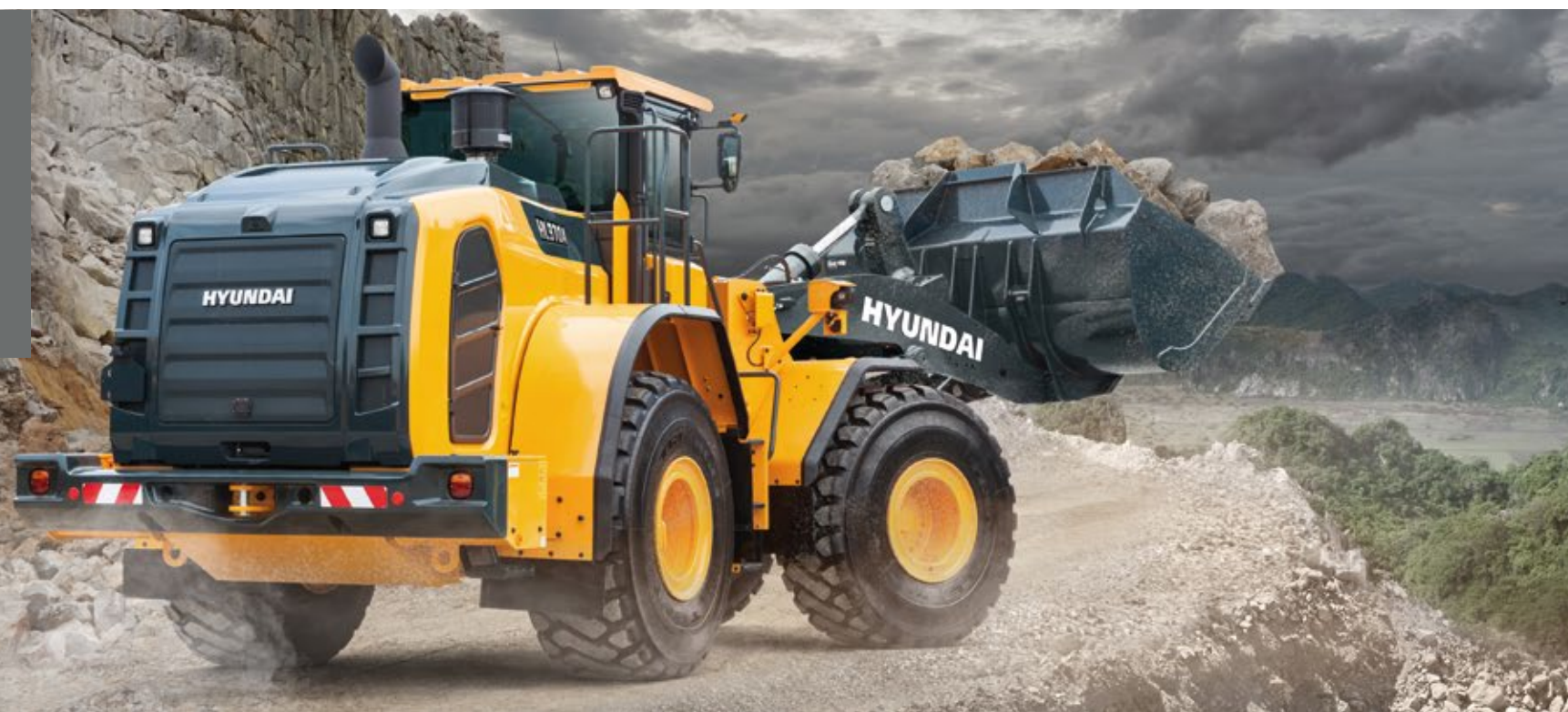
The new Smart Power mode adjusts engine RPM in heavy load work like digging to save fuel without compromising on performance. The technology also achieves an optimal balance between traction and breakout forces.
