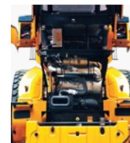
The **engine hood is fully retractable** and can be **opened electrically** for easy access to the sealed engine room and cooling room. The engine room is designed to prevent the possibility of fire caused by the inflow of foreign materials.
