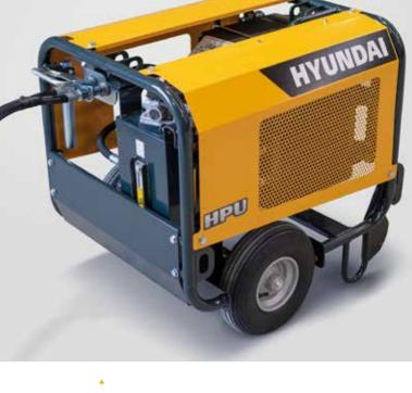
In addition to the integrated diesel engine, the HX10A can be powered by an optional electrohydraulic unit for low noise, zero-emissions operation. This makes it the ideal choice for work indoors or in sensitive environments. The generator is simply connected to the undercarriage and has no impact on machine handling or performance, even in breaker operation.
