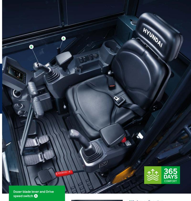
Two-handed operation for skilful and efficient levelling with drive mode changeover on the drive lever handle.
