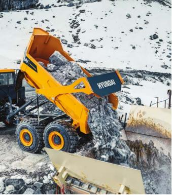
The optional heated body prevents frozen material sticking to it, enabling quicker and
