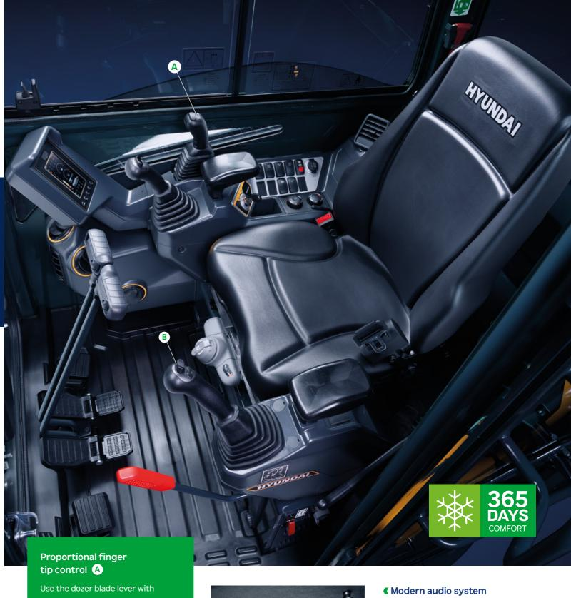
Use the dozer blade lever with fingertip control to define the perfect driving speed when grading.
